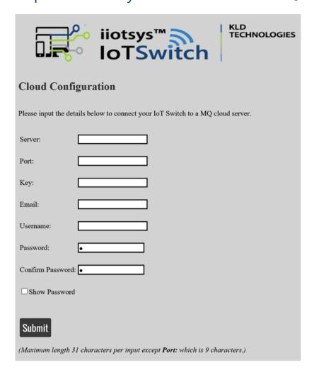
The ioTSwitch can also be controlled from cloud services, custom home automation systems that support MQTT protocol. The requirement for this section is both local Wi-Fi network and internet access for any related cloud services.
