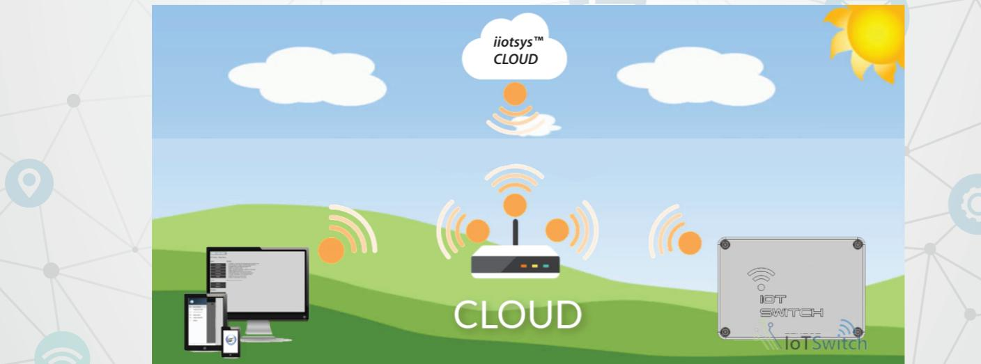
The iiotsys™ IoT Switch connects to a secure cloud platform using your Home or Office Wi-Fi router and waits for messages that control it. The **Mobile App** loaded on your phone securely connects securely to the **Cloud platform** using either your home, office or 3G/4G/LTE internet connection and passes control messages to your iiotsys™ IoT Switch. This allows control of connected appliances and electronic devices from your home or office and from the internet.
