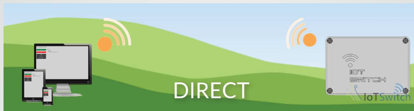
Where there is no home or office Wi-Fi network the iiotsys™ IoT Switch acts as an access point and can be controlled directly by connecting to it and using its local built in **Web interface**, this allows control of connected appliances and electronic devices where there is no existing network.
