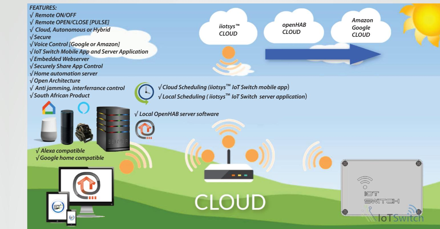
The iiotsys™ IoT Switch integrates seamlessly into openHAB home automation server, this allows for creation of control panels throughout your home or office and can be extended to enable voice control with Amazon Alexa or Google Home. This allows control of connected appliances and electronic devices, as in the cloud mode, but now extends control to include all the benefits of home automation server controls and rules.
