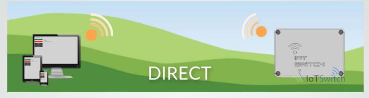
Where there is no home or office Wi-Fi network the iiotsys<sup>™</sup> IoT Switch acts as an access point and can be controlled directly by connecting to it and using its local built in **Web interface**, this allows control of connected appliances and electronic devices where there is no existing network.
