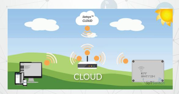
The iiotsys™ IoT Switch connects to a secure cloud platform using your Home or Office Wi-Fi router and waits for messages that control it. The **Mobile App** loaded on your phone securely connects securely to the **Cloud platform** using either your home, office or 3G/4G/LTE internet connection and passes control messages to your iiotsys™ IoT Switch. This allows control of connected appliances and electronic devices from your home or office and from the internet.
